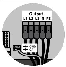
3.3.3 Check output connections, HV-board. Only in cases of no continuity of the EV gun or no 12Vcc in the CP or with or in cases of intermittent charges.
