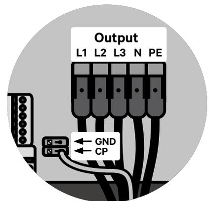
3.3.3 Check output connections, HV-board. Only in cases of no continuity of the EV gun or no 12Vcc in the CP or with or in cases of intermittent charges.
