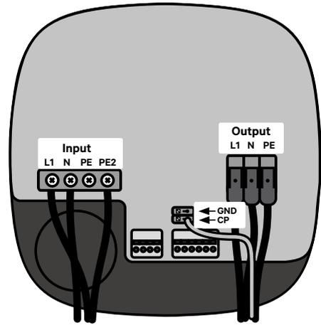
3.2.3 Measurements on the power supply of the charger.
